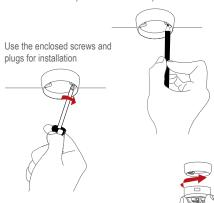
2. Mount the heat alarm to the base by using the smart clip-on-ceiling mechanism. After mounting, test the heat alarm by pushing the test button on the side and get an alarm signal.
