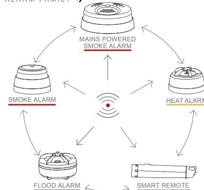
All CAVIUS interconnected alarms within the **WIRELESS** ALARM FAMILY can be added to the system as they run on the same frequency and use the same
